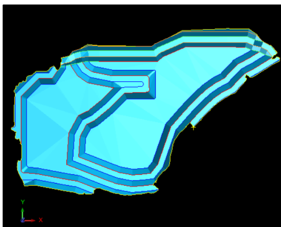
Gambar 2. Desain mine sequence area selatan Pit Hill16 bulan April
