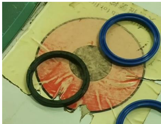
Gambar 1 Kondisi kerusakan mechanical seal .
