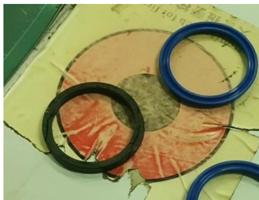
Gambar 1 Kondisi kerusakan mechanical seal .
