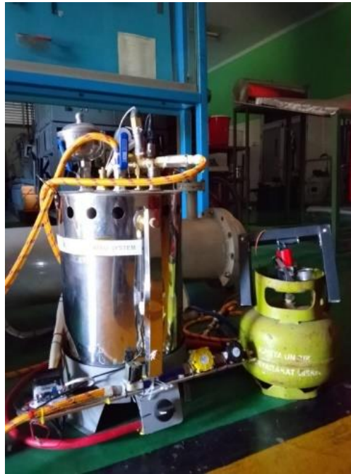
Gambar 1. Prototype steam plant dalam sistem Vessel to Grid (V2G)
