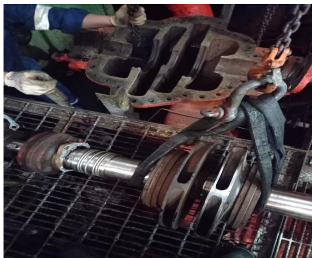
Gambar 6. overhaul shaft cargo oil pump .Sumber: Penulis (2024)
