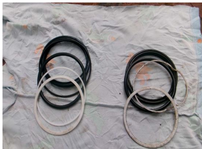
Gambar 4. Renew O-ring dan Oil Seal
